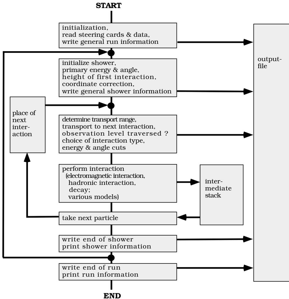
Figure 2: Simplified flow diagram of CORSIKA.
