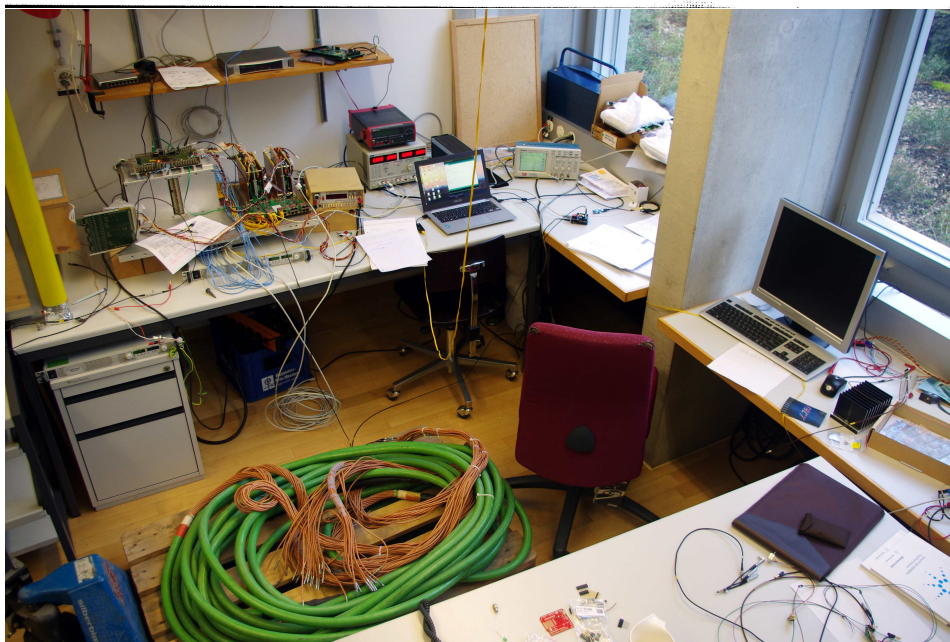
Figure 5.3: Top: The signals before and after the 44m cable. Bottom: Test set-up in the ETHZ basement next to a naked working sector of the FACT camera electronics
