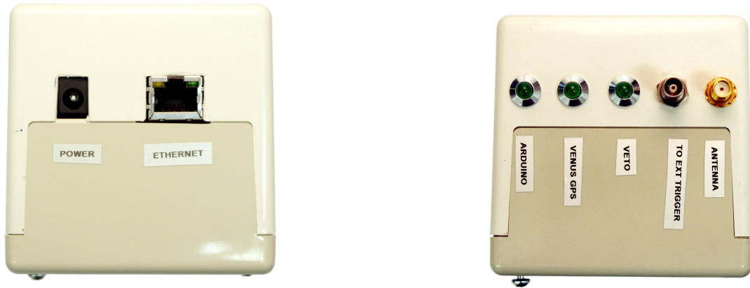
Figure 2.2: The FACT GPS module sides
