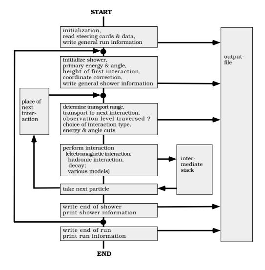
Figure 2: Simplified flow diagram of CORSIKA.
