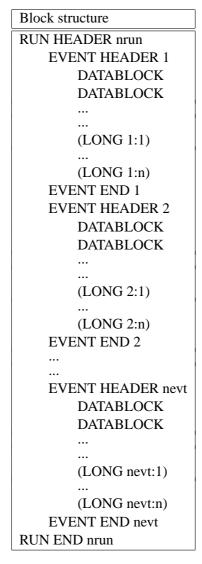
Table 6: Block structure of the particle and Cherenkov photon output files. (The LONG blocks eventually occur only in the particle output file.)
